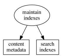
Using celery\_haystack, index-management tasks are triggered by "save" signals on the ORM model that the index is based on. Because the crawler is NOT using the ORM, inserts/updates/deleted by the crawler do not automatically trigger these tasks. Instead, scheduled jobs compare content hash fields in the drawler's database and the metadata to detect differences and dispatch metadata updates appropriately.
