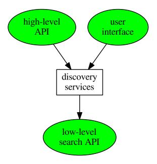
The disco services are implemented as python/django applications, run in a stateless wsgi container (gunicorn) behind a reverse proxy (nginx). Django is used to produce both the user interface (responsive web) and high-level API (REST).
