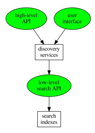
In the above diagram, green ellipses represent interfaces. The colour green is used to indicate that the items are open for public access.
